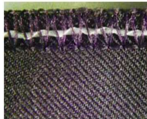
Coats fusion hemseal is channelled within the overlock stitch formation.
