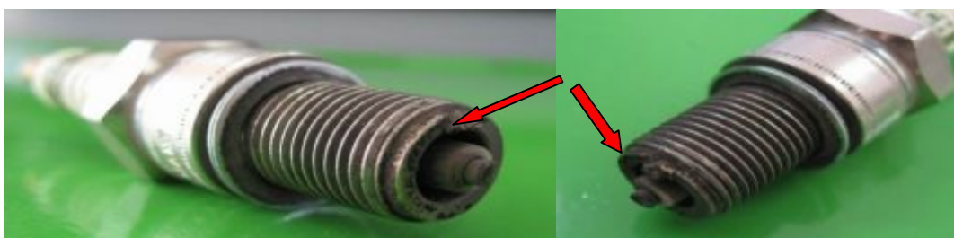
Fig. 9. Failure of removing the spark plug side electrode
